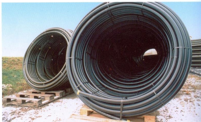
Fig. 9-1: Reeled pipes made from Hostalen materials
